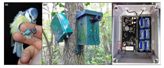
**FIGURE 1** (a) An example of a PIT tag, here embedded in a leg band and attached to a blue tit. (b) Waterproof box containing the radiofrequency identification (RFID) logger mounted on a tree (left side) with antennas placed in front of the nest box opening. (c) Inner side of the RFID box, containing the battery holder, RFID data logger circuit, and a 1 GB memory stick for data storage and programing
